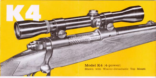
accuracy. Lenses are hermetically sealed and cemented in their cells, air-tight, vapor- and moisture-proof. No loose lenses. All threaded metal joints are sealed with Neoprene O-rings — a positive compression seal. This is a new development in scope sealing, available only in Model K Weaver-Scopes. All Weaver K Models are nitrogen filled to prevent fogging.
