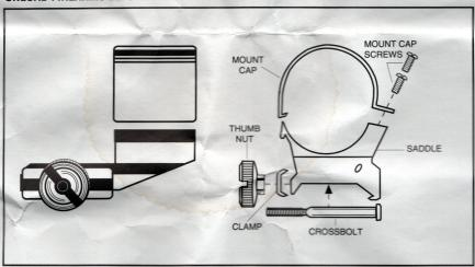
A Weaver Extension Ring with a Detachable Top Mount is necessary for use with large objective end scopes, variable power scopes, or the newer compact scopes.
