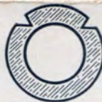
Shows dovetail grooves in rifle.
